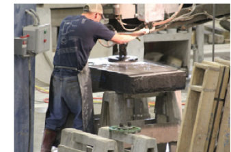
A worker uses a stone grinder that applies water at the work surface to reduce silica dust levels in the air.
